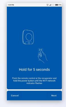
2. Point the remote control at the recuperator and hold the "ON/OFF" button until the blinking Wi-Fi symbol appears on the display. Click "Next".
