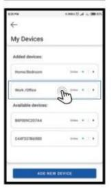
To edit the device name, press on the required recuperator name (e.g. «Work / Office»). Press «Edit» on the device information screen and enter a new name. Press «OK».
